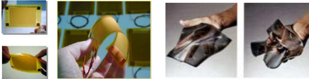
Figure 1 MFC Actuator (left) and Metal Rubber sensor material (right)
