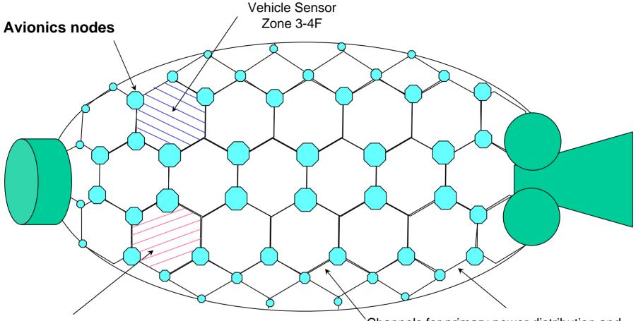
Flexible Solar Panels embedded in outer skin material Channels for primary power distribution and thermal control infrastructure
