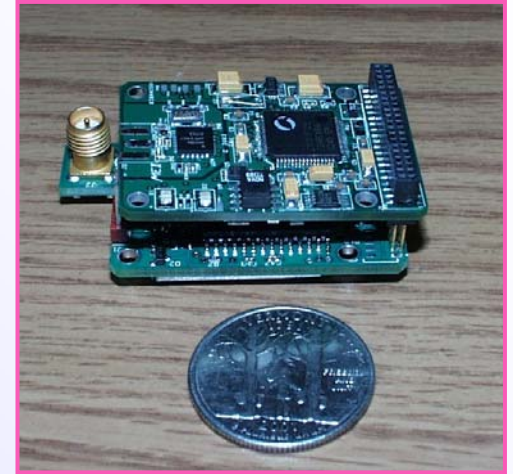
Example of Remote Station for H2 (sensor not shown)
