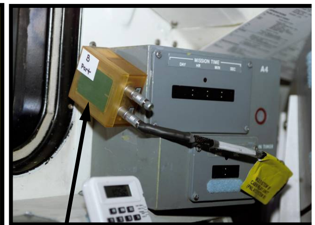
Cabin Relay Unit (A & B) communicates with wing Relay Unit A or B and sends data to laptop
