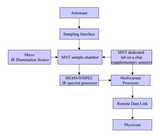
Fig. 3: Detail of MNT/IOSPEC diagnostic system.
