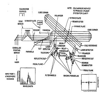
Fig. 7: Schematic of typical FT-IR system used in space (after [14]).
