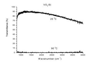
Fig. 6: FT-IR optical transmittance of MPB/INRS  $VO_2$  on Si in the insulating (29°C) and metallic (95°C) states.
