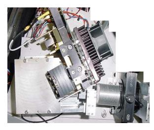
*Fig. 4: Photograph of current IOSPEC module weighing under 2 kg including input optics and cooled detector array.*
