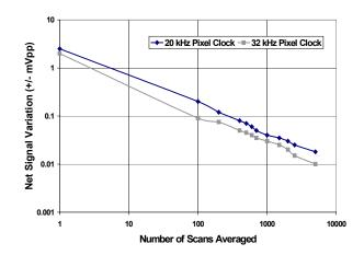
*Fig. 5: Variation of typical noise for 256 pixel multiplexed PbS array at 260K with the number of scans in active smart average.*
